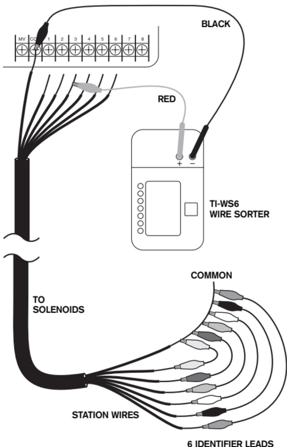
One end of the lead clips to each station wire to be tested, the other clips to the common ground
