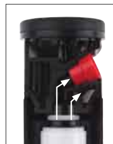
Upper arrow: Water flowing to main orifice Lower arrow: Water to secondary orifice.
