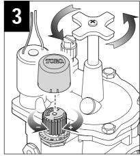
With the valve operating, turn the flow control handle to the left for maximum flow. Remove the regulator cover. Turn the knob left or right until the indicator aligns with the desired downstream pressure. Install the regulator cover when finished.
