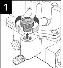
**Note**: During installation of the EZReg module, the irrigation valve can remain pressurized but should not be operated.
