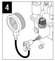
4. Optional – To verify downstream pressure, attach a Toro pressure gauge (model 995-51) to the test valve stem as shown. With the valve operating, read the indicated pressure on the gauge and adjust as necessary. Install the regulator cover when finished.
