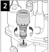
2. Install the EZReg module. Tighten 1/16 turn after the hexagonal flange contacts the valve body.
